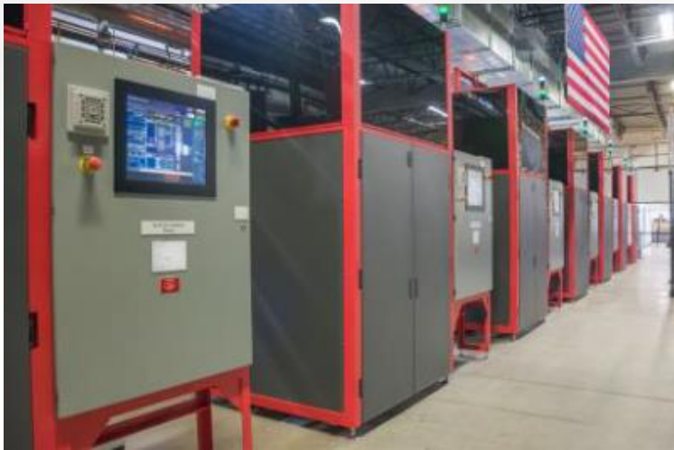
Advanced automated SiC crystal growth systems
